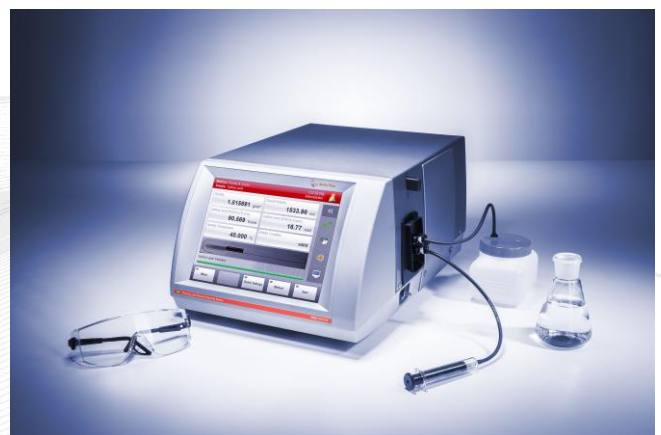
Figure 2: Filling DSA 5000 M with a glass syringe
